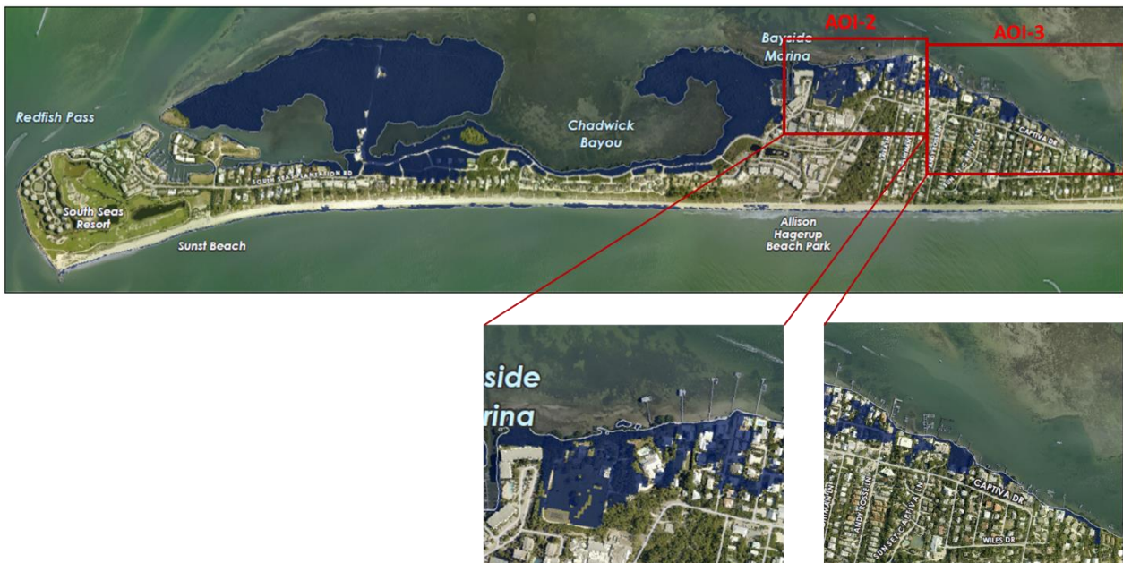
Figure 2. AOIs-2 and 3 are located on a bayside promontory that is openly exposed to Pine Island Sound. The coastal changes orientation from north to south so will be more exposed to fetch waves from different directions.
