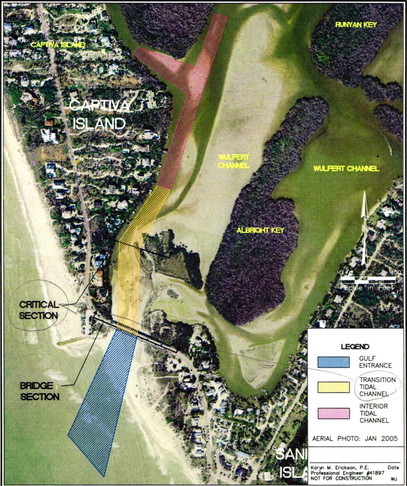
FIGURE 3-1 GENERAL PLAN VIEW OF CHANNEL ALTERNATIVES Blind Pass Restoration Lee County, Florida
