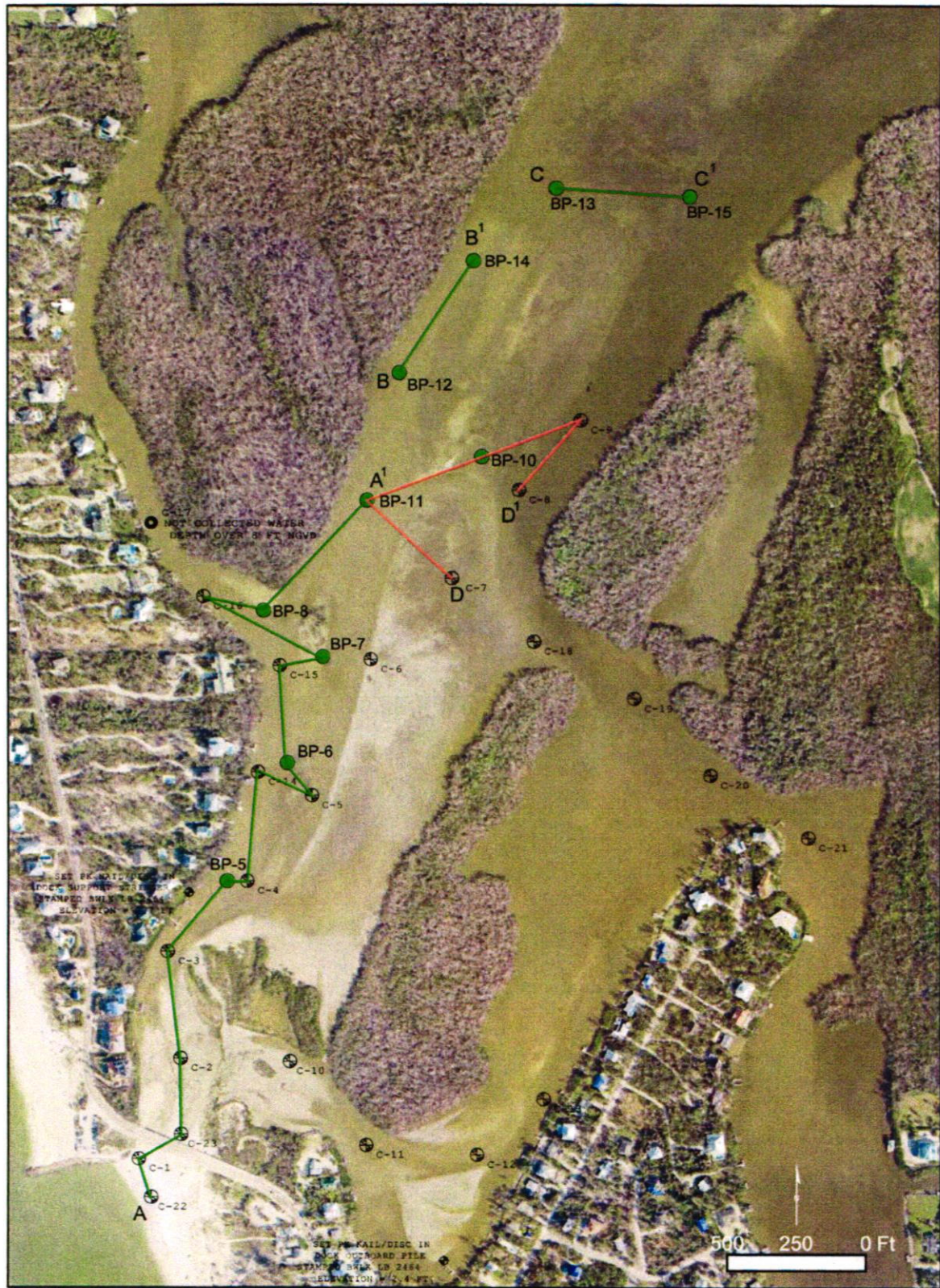
Figure 2-21 Plan view of core locations and geologic cross sections within the study area.
