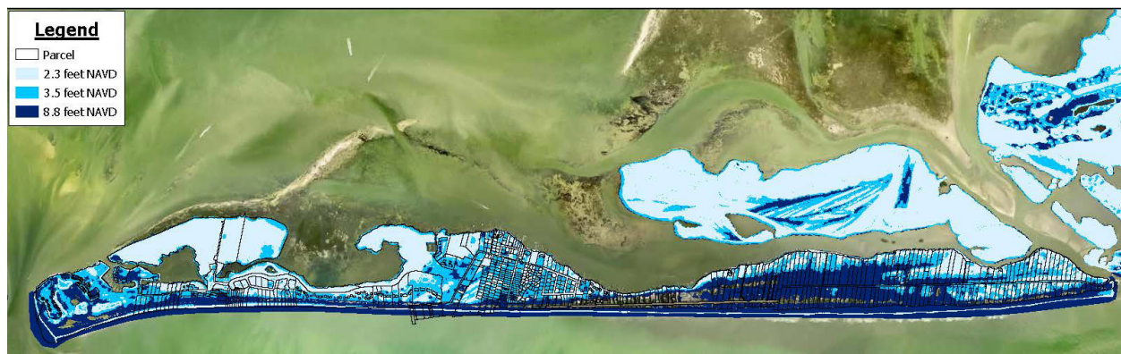
Figure 15. Parcel Inundation Map for Inundation Tipping Point Scenarios.
