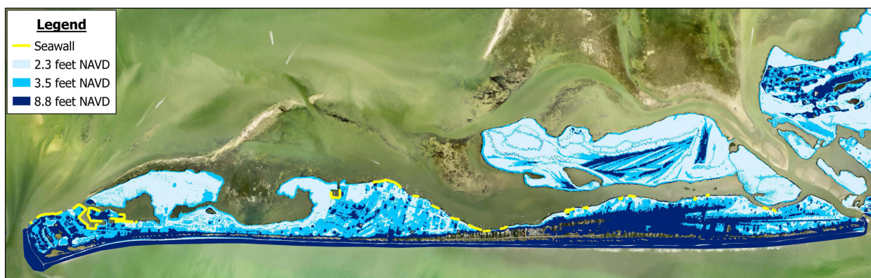
Figure 25. Seawall Exposure Map for Inundation Tipping Point Scenarios
