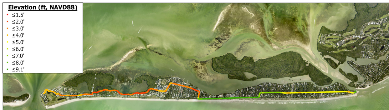
Figure 38. Captiva Evacuation Route Elevation
